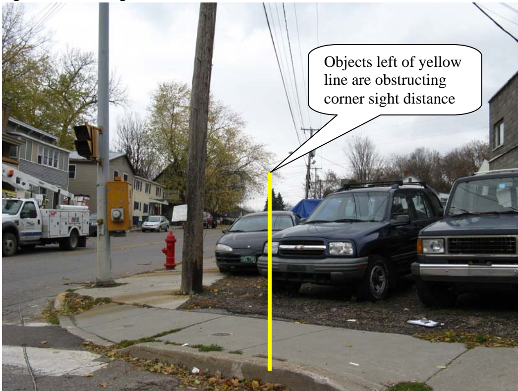
Figure 1: Corner sight line of northeast corner
